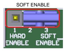
Use Hardware Enable to keep the driver enabled all the time. Set of jumpers as shown in the image.
