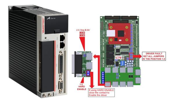
5.2 Diagram of connection with input signals Differentials C74 and C76.
