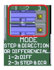
If not use the differential signal for STEP & DIR, set jumper as show in the image.
