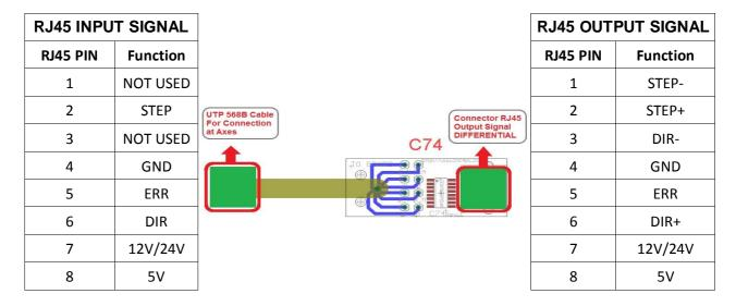
The output signals of STEP and DIR are differentials.
